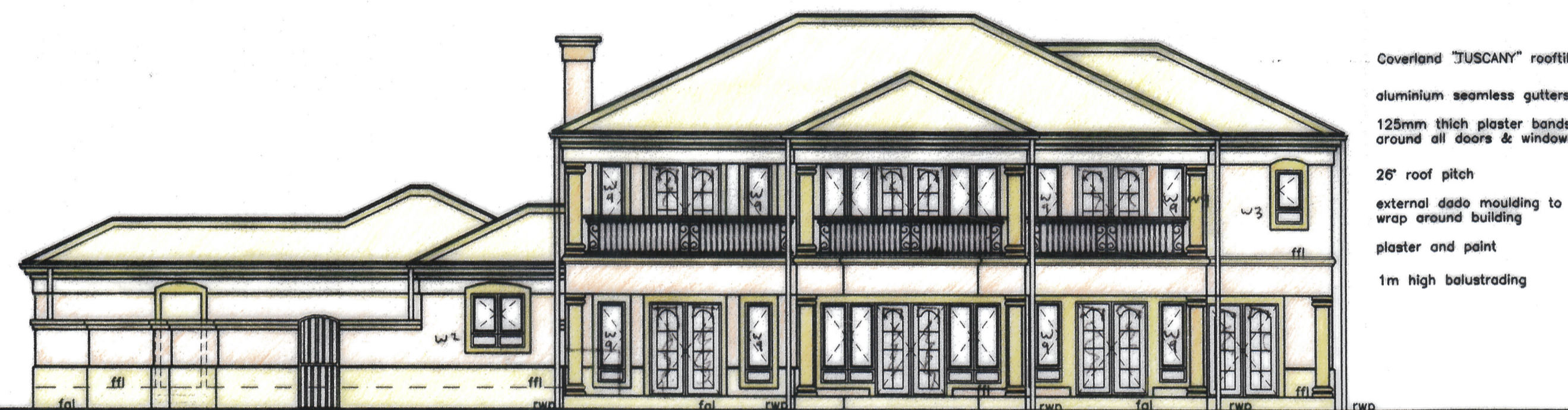
NORTH WEST ELEVATION
